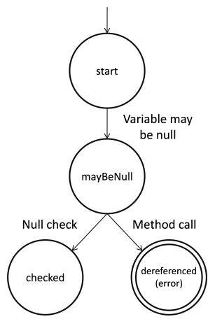
The Control Flow Analyzer sets the FSM state to mayBeNull when it observes that the JSP code assigns a value to the incomingParameter variable. At this point, the code has not yet verified that the variable's value is not null.
