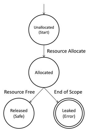
First, the analyzer allocates a separate FSM for each object. Then, the analyzer sets the object's initial state as unallocated before code allocates the object. After code allocates an object, the analyzer updates the object's FSM state to the allocated state. Then, the analyzer examines all codepaths that are within the object's scope.
