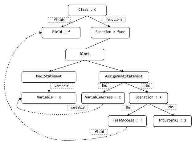
As an example, the following query matches any assignment in the program in which the location being written to is a local variable and the expression for the value includes a read of a field, which belongs to the same class as the class in which the function appears. This matches the previous example code. Unlike the query in "Example 2" on page 34, it does not include constraints on names. It is general enough to match similar code patterns in other parts of the program.
